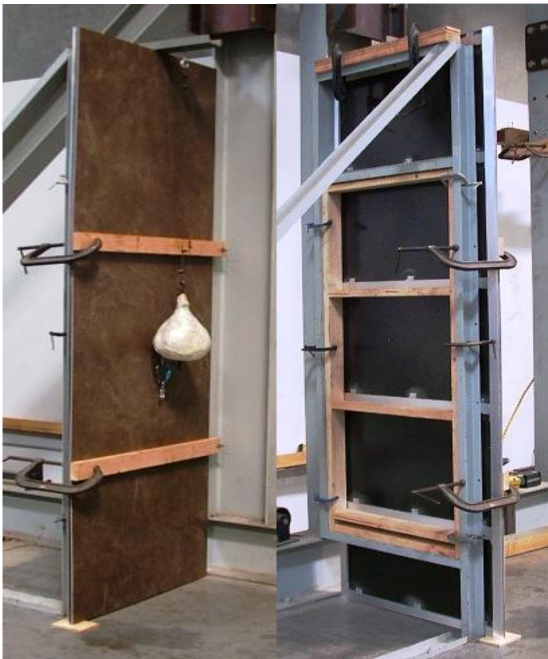
Photographs 1 and 2 Impact Test Set-up Impact Side and Back Side
